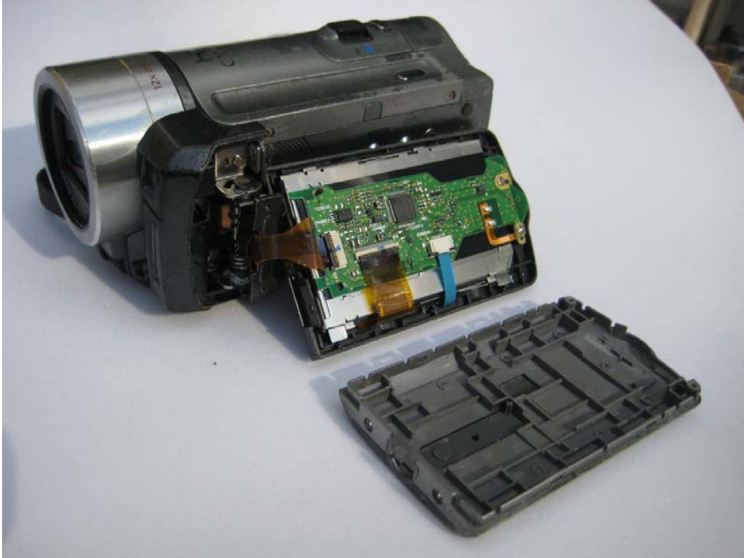
Cover outside screen removed.
