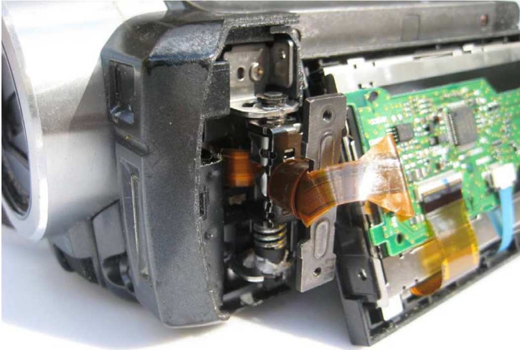
Inside view from lens end. Covers removed from part of case containing ribbon cable.
