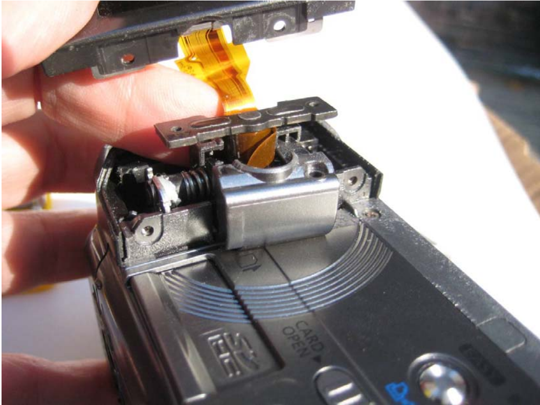
The hinge is open and both pieces of ribbon cable cover are ready to snap together.
