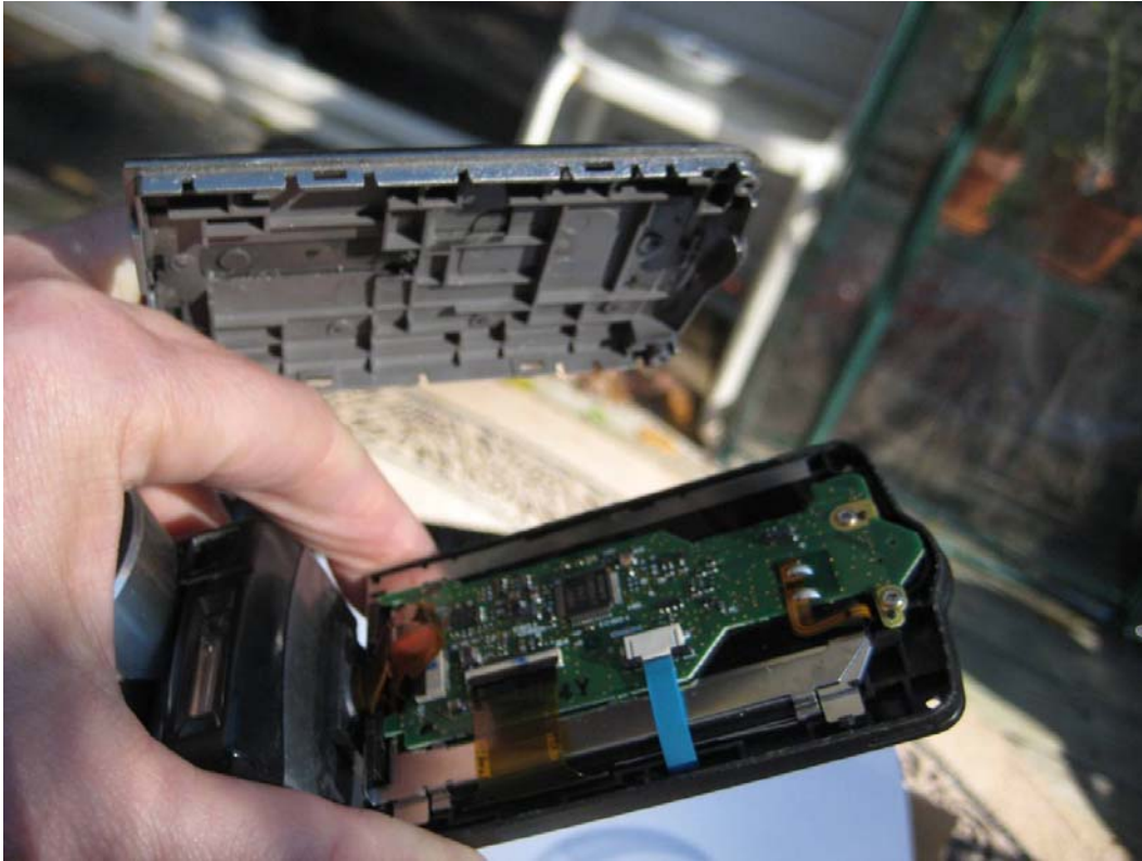
Outer cover of screen is ready to replace.
