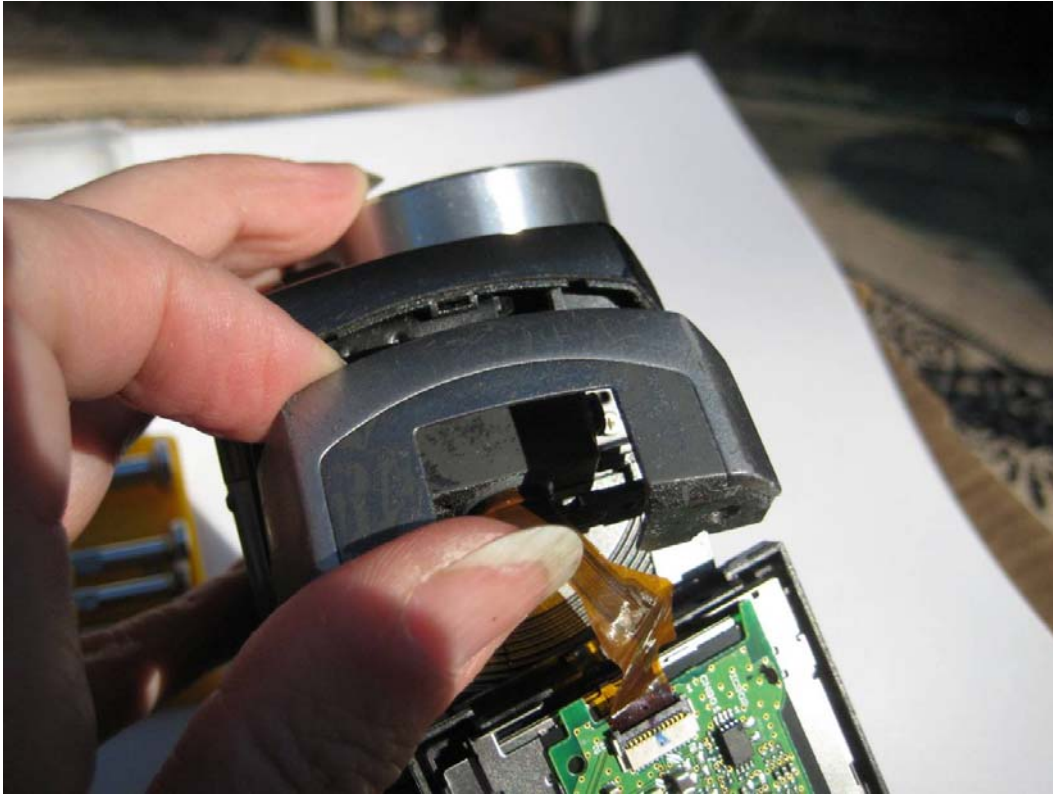
Outer cover is ready to slip under the edge near the lens on the case.
