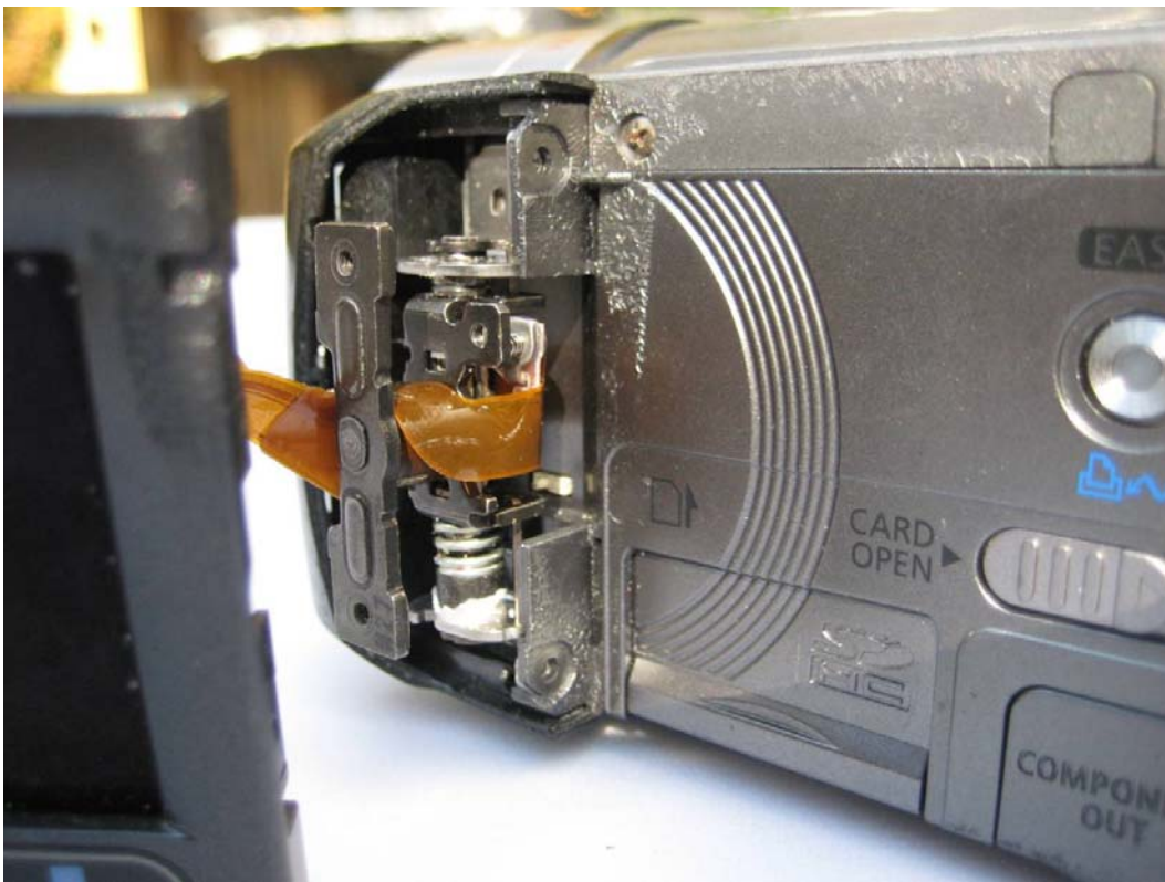
Inside view from viewer end. Hinge snapped down over ribbon cable.
