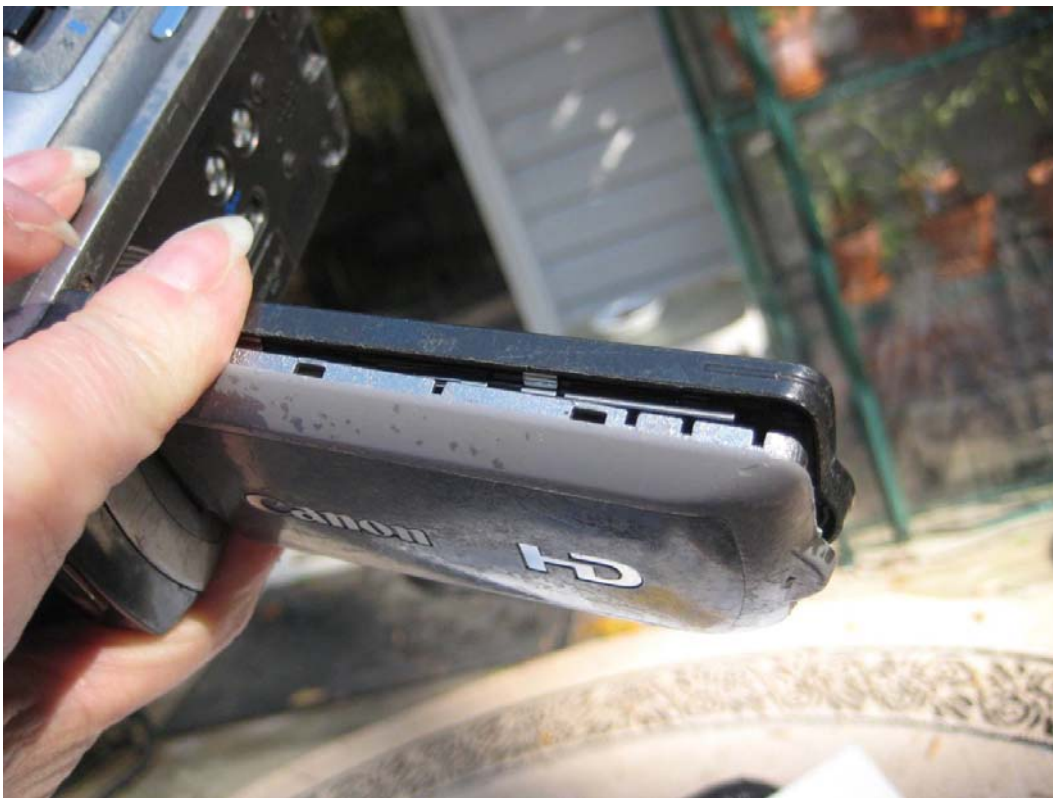
Outer cover of screen ready to snap into place.
