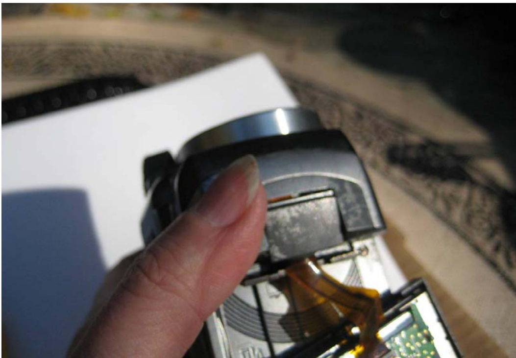
Outer cover snaps down gently over the ribbon cable covers. Check to make sure it's in the slots behind the hinge.
