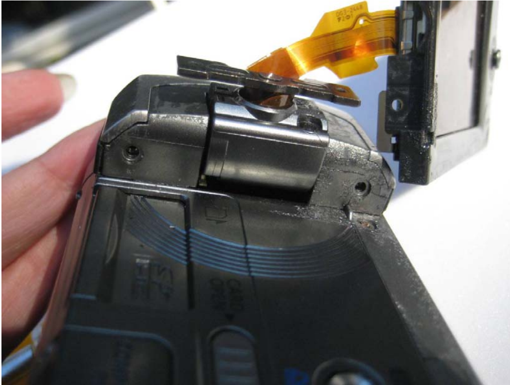
Ready to replace the 2 screws to secure the covers in place.
