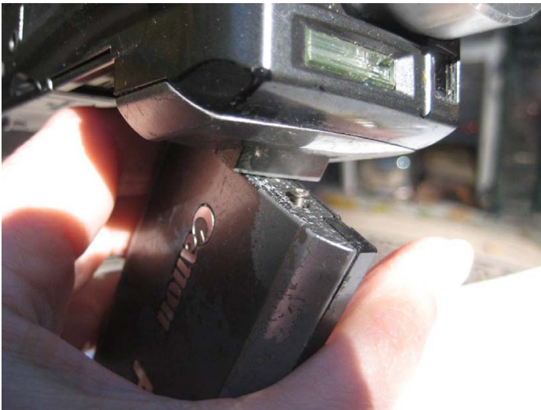
Turn opened screen 90 degrees and replace screw on each side of hinge.
