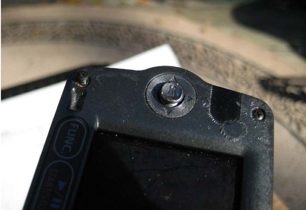
Replace screws at each corner to the left of screen.
