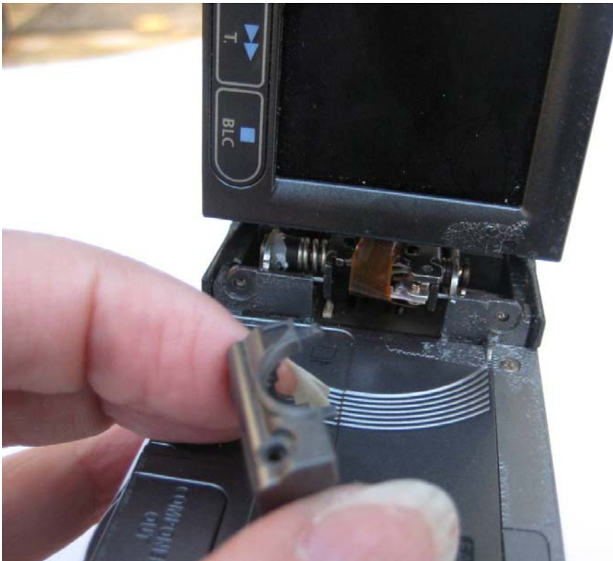
The inside piece with the screw hole will slide over the ribbon cable under the screen.
