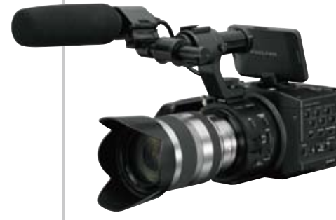
A-mount lens with the LA-EA1 adaptor
