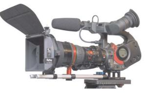
The XLAnamorphic can also be ordered with a Light Weight Support system instead of the system support bracket, to allow sunshades and other accessories to be used in conjunction with the adapter (Product Code: OTDVXLANALWS)
