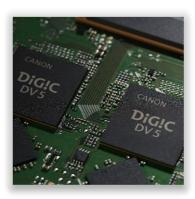
Two DIGIC DV5 image processors boasting a high data processing power are incorporated expressing a wide range of image expressions such as 4K movies with a high bit rate of 410 Mbps.
