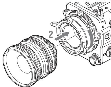
**To attach an ARRI\* LDS lens or Cooke/i lens**
